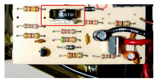
It's actually quite easy to access the pot just by putting your fingers underneath the board. You can get to the pot from any direction EXCEPT where access is blocked by the chassis or a major power supply component, such as the power transformer or the main filter capacitor. There are no dangerous voltages present under the board but you should avoid the exposed 120VAC primary power input connections and the power switch that are usually located on the other side of the supply.
